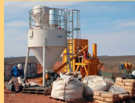
Automatic slurry mixing system SCC 40 in Kleinzee, South Africa
